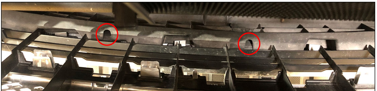
FIGURE 2 – Lower Grille Retention Clips (only 2 of 5 pictured)
