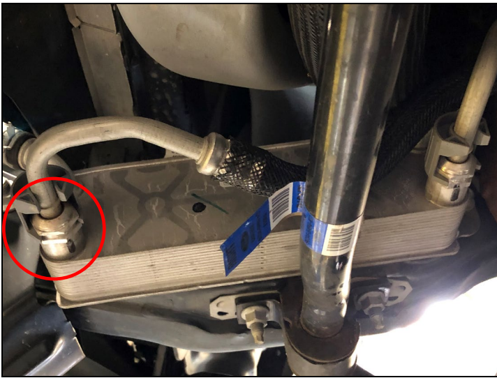
FIGURE 15 – Stock Trans Cooler – Outlet Marked
