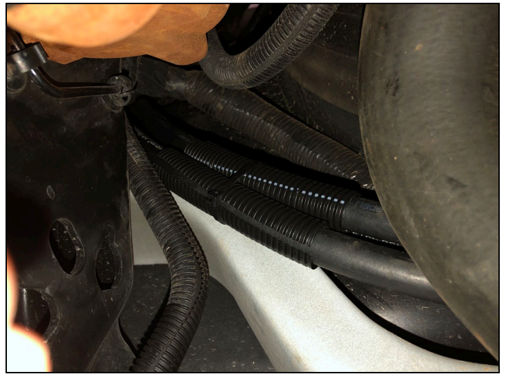
FIGURE 21 – Protective Loom and Cable Tie on Hoses
