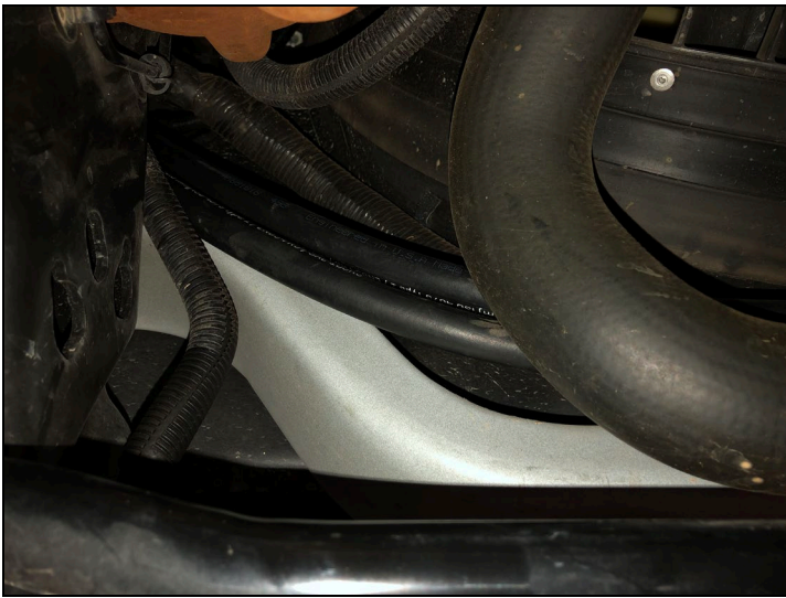
FIGURE 20 – Cooler Hoses Tucked Above Core Support
