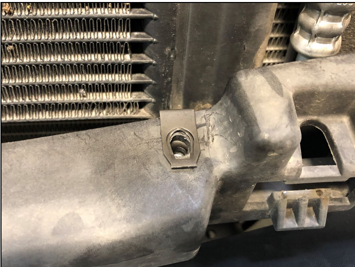
FIGURE 6 – Hole Drilled & Clip Capture Nut Installed
